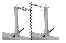
2. Identify suitable end anchors. This includes stanchions, heavy duty D-rings, suitably drilled I-beams, anchor slings, etc.
